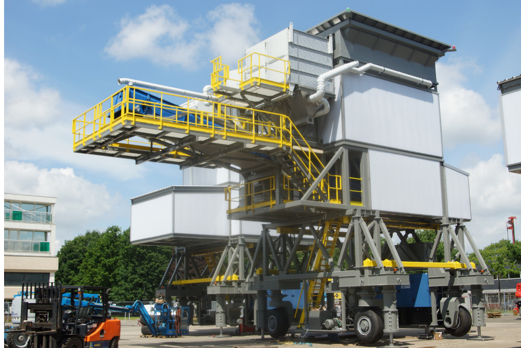
Mobile scales: Meyland initially builds every hopper in Belgium, tests it and only then ships it to the respective country of destination.
