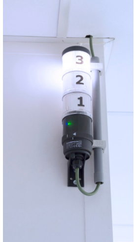
Image, left: A signal tower in the canteen indicates whether there is a machine fault, and, if so, in which area of the workshop.
