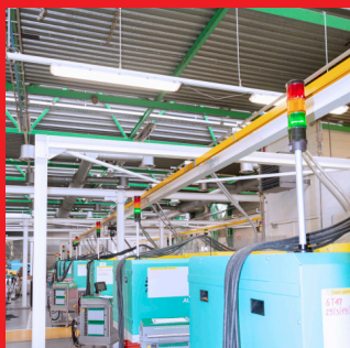
Each machine already had a WERMA signal tower, which was quickly and easily kitted out with a SmartMONITOR module.
