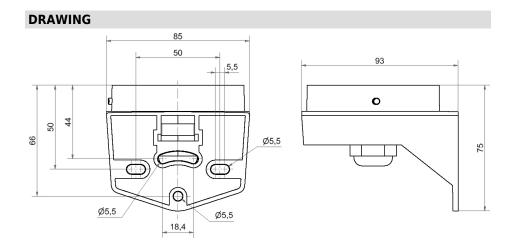
For additional installation and mounting information, refer to the appropriate user guide at www.werma.com. This printed copy is for information only and is subject to alteration.
